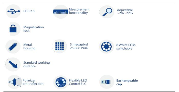
The AM7115MZT is part of the universal range and with its standard working distance and wide magnification range from 20 - 220x, it is suitable for a wide range of applications. Because of the built-in polarization filter this model is ideal when working with shiny or reflective objects such as metal, plastic, glass, jewelry, electronics, etc.
